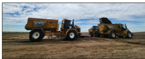
METROGRO® Cake is loaded into a TerraGator.
