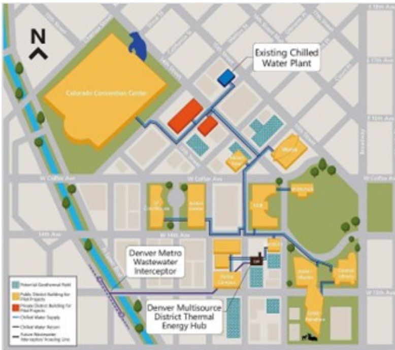
Twelve Denver-owned buildings around Civic Center will serve as the initial, scalable Ambient Loop pilot area by leveraging Xcel district-chilled, water piping (Image credit: Energetics Consulting Engineers, LLC).
