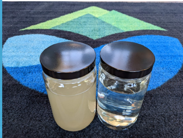
NTP untreated influent (left) compared to treated effluent (right) in May.
