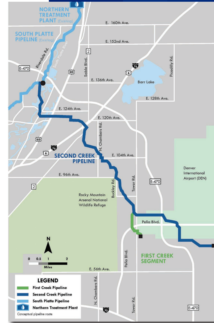
Second Creek Pipeline proposed alignment
